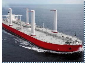
REEL in partnership with CRAIN is developing an auxiliary wind propulsion device for cargo. This system consists of a thick and solid wing, equipped with a rear flap. An internal fan makes it possible to suck up the boundary layer and achieve an extremely high coefficient of lift. The wing thus sucked produces force and propels the ship in combination with the main engine.
